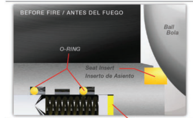
Fire safe packing / Empaque fire safe
